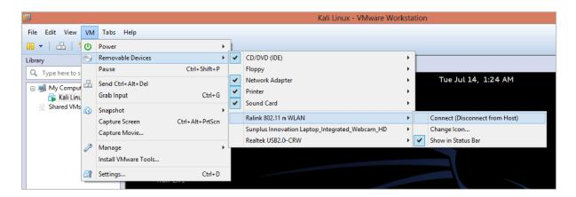
Here, Windows is the host machine for any VMWare OS. To connect and access Alfa card inside of Virtual Machine we have to disconnect it from the host system(Windows).
