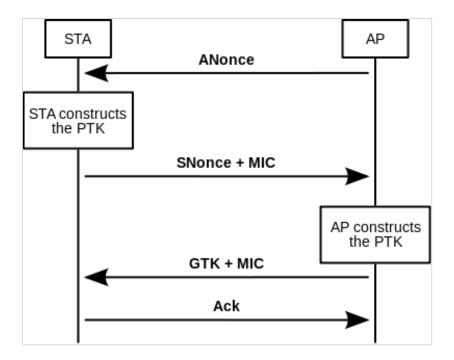
The actual messages exchanged during the handshake are depicted in the figure and explained below (all messages are sent as EAPOL-Key frames):
